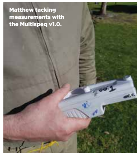
The prototype MultispeQ used by the team of global beta testers that was 3D printed.
