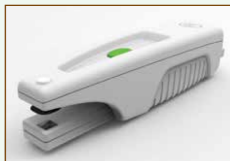
Figure 8B: The MultispeQ V1.0 sensor which links to a mobile phone via a PhotosynQ app.
