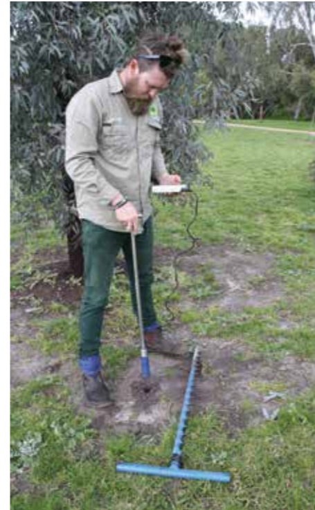
Figure 9B: Measuring soil moisture with a moisture probe.
